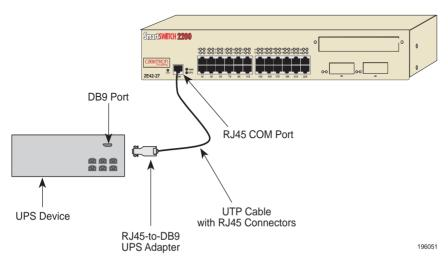
Figure 5-2 Uninterruptible Power Supply (UPS) Connection
